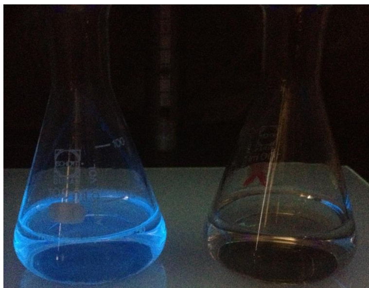
Figure 5-1: A typical example depicting the fluorescent ability of quinine sulfate in sulphuric acid solution (left) which is quenched by the addition of hydrochloric acid (right).
